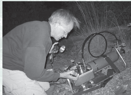
Kevin Rice with a pressure chamber measuring water potential at 3:00 a.m. in the morning.
